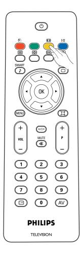
Press this button to display a list of available display formats. Available display formats are determined by the type of signal you are receiving. To choose the display format you prefer, press the FORMAT button repeatedly:
